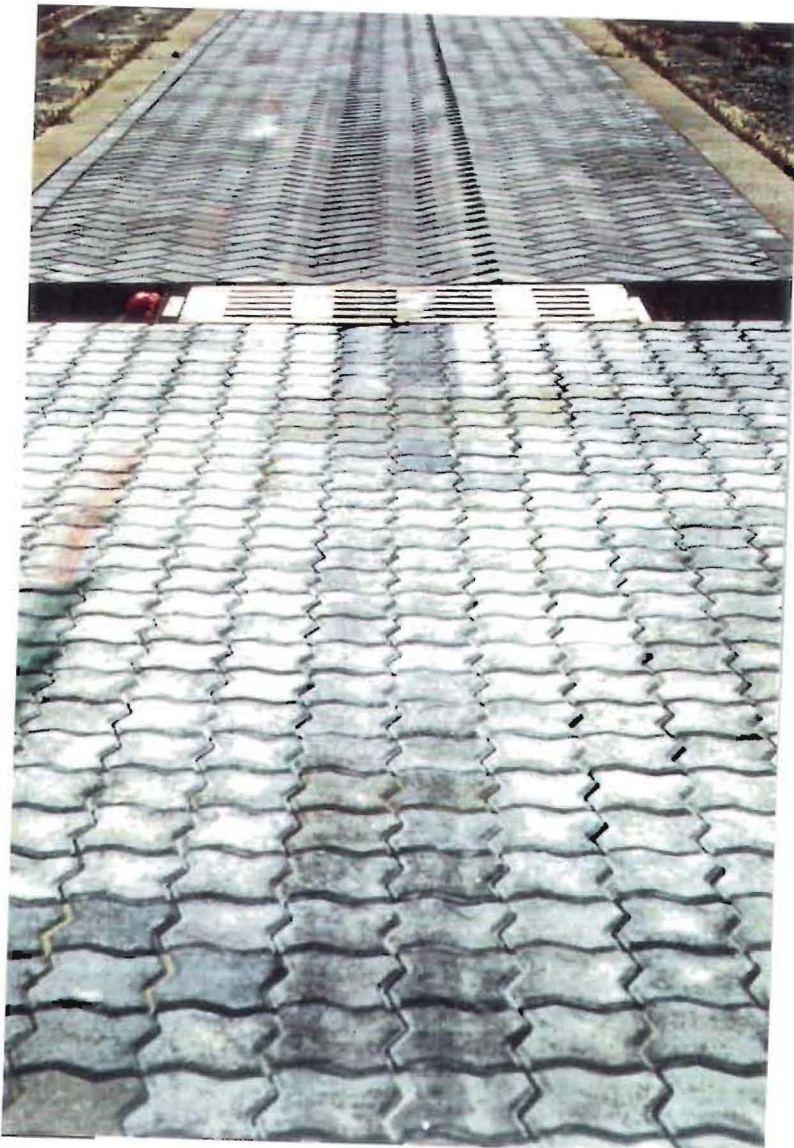
UNI-ANCHORLOCK® paving stone section, showing no deformation after NASA test trial runs, Spring 94
